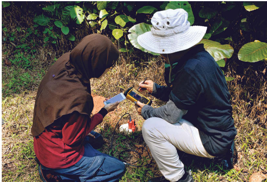
A seismometer being installed by researchers Mark Lim and Dannie Hidayat. A total of 88 seismometers were deployed islandwide to detect seismic events and background noise. They are sensitive enough to detect even the slightest bit of noise or shaking. PHOTO: JANIATOR TULIUS, EARTH OBSERVATORY OF SINGAPORE, NTU
